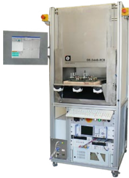
Automatic test systems for testing of electrical and radio-relevant parameters
