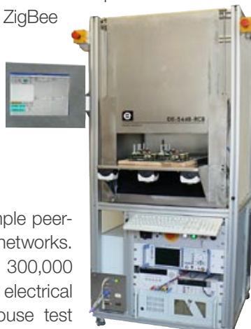
Automatic test system for testing of electrical and radio relevant parameters
