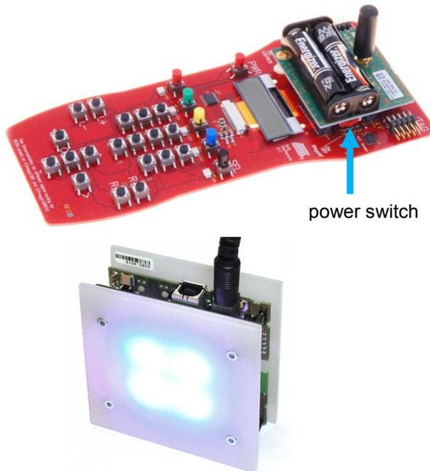
1. Connect the SMA stub antenna to the connector on the RCB128RFA1 board.
